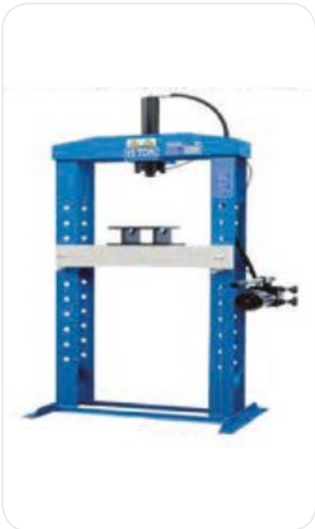
Hydraulic 20 Ton Floor Press with Gauge Hand Operated with 2 Speed Pump 200mm Ram Stroke 1020mm max working Range 510mm Bed Width including V-Block
