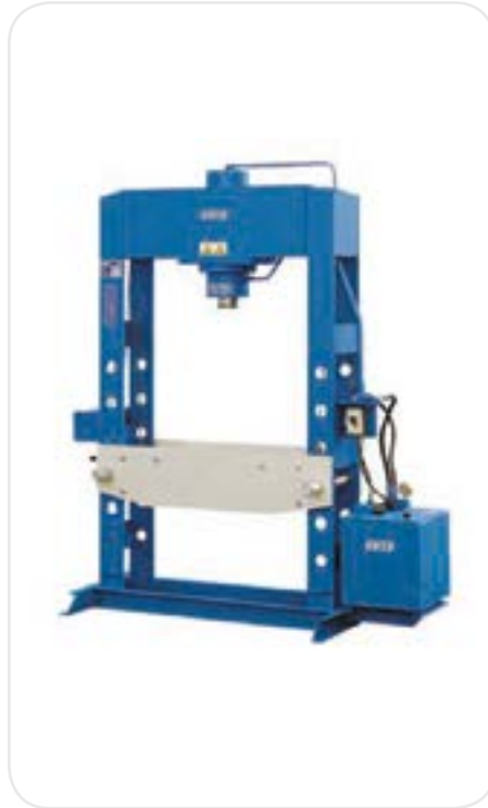
Hydraulic 100Ton Floor Press with Gauge Electric 1 Speed Pump 380v | 310mm Ram Stroke 1055mm max working Range 1010mm Bed Width including V-Block
