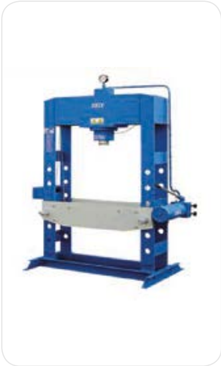
Hydraulic 50 Ton Floor Press with Gauge Hand Operated with 2 Speed Pump 190mm Ram Stroke 1135mm max working Range 335mm Bed Width including V-Block
