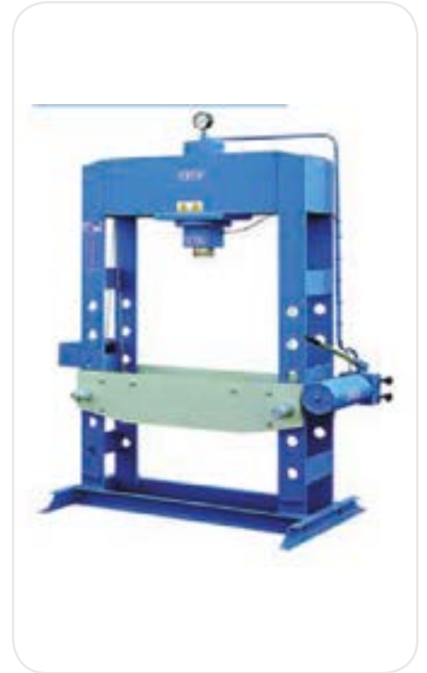
Hydraulic 100Ton Floor Press with Gauge Hand Operated with 2 Speed Pump 215mm Ram Stroke 1055mm max working Range 1010mm Bed Width including V-Block
