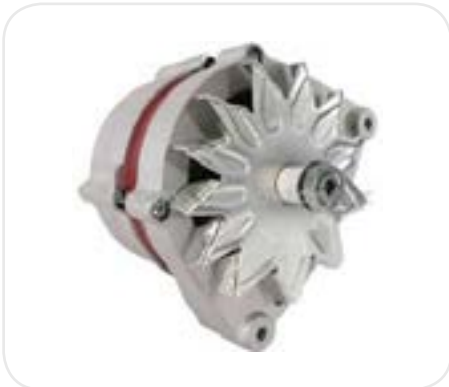
Iskra & Bosch Type External Fan 24 V | 55 amp | 2 x 56 ear HDE00013
